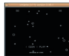
Atari's vector scan Asteroids delivered far higher resolution than traditional raster-based games.
