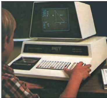
Commodore's PET 2001 was the first all-in one personal computer, but the fiddly key grid was bad news for touch-typists.
